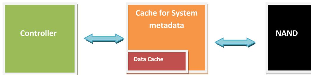
The SFCT allows incoming host data to make a “pit stop” in cache and then pushed into the NAND media immediately, as long as there is no bottleneck on the flash interface. When the flash interface becomes jammed due to particular file sizes (random 4K), cache are being treated as “organizers”. The incoming write data will be consolidated into groups before written into flash to improve the write amplification and acknowledge host only when the data is fully committed to the NAND media.
