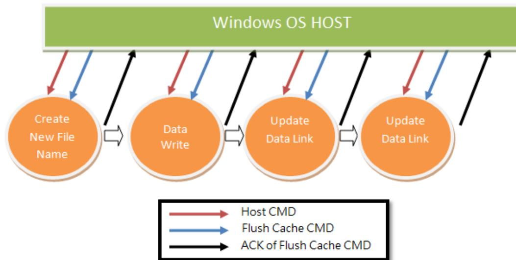
The FLUSH CACHE CMD following each important stages of a given task allows the OS to re-build system table / file system table (For Windows, CHKDSK, for Linux, FSCK) upon return from power fail.
