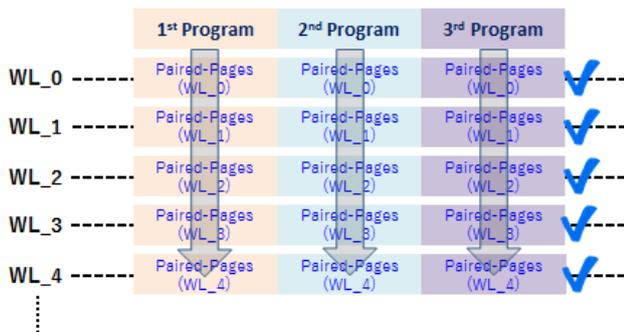
Fig.3 Programming Operation of TLC Flash
