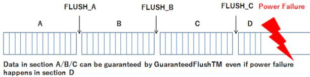
**Fig.5 Timing of Triggering GuaranteedFlush™**
