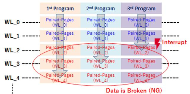
Fig.4 Power Loss during Data Programming
