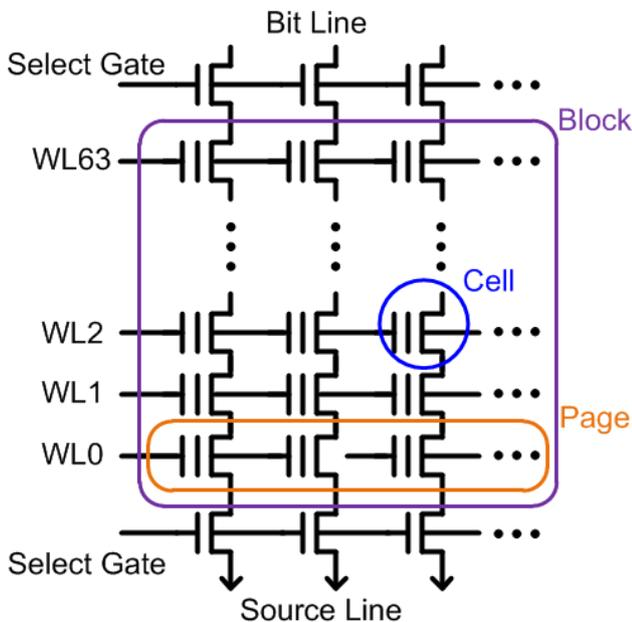
Fig.1 NAND Composition in Transistor Level
