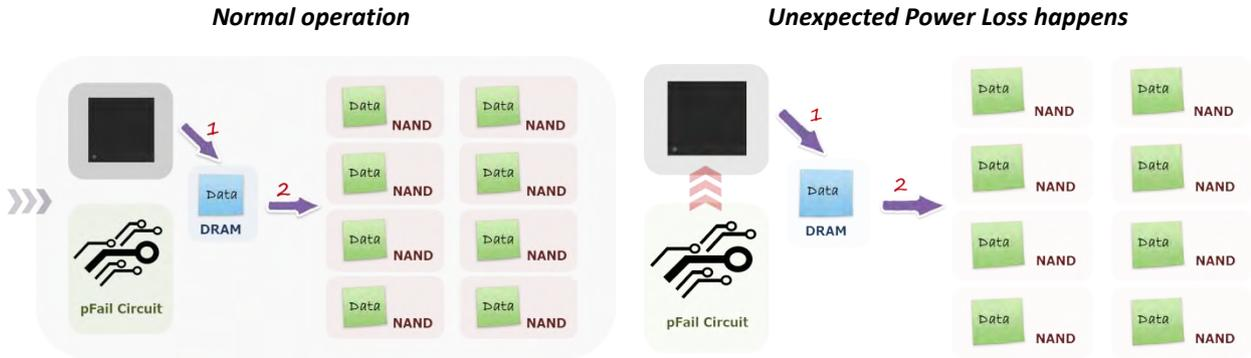
*The SSD is powered by the power supplied from host side, and the capacitors in pFail circuit is charging up.*
