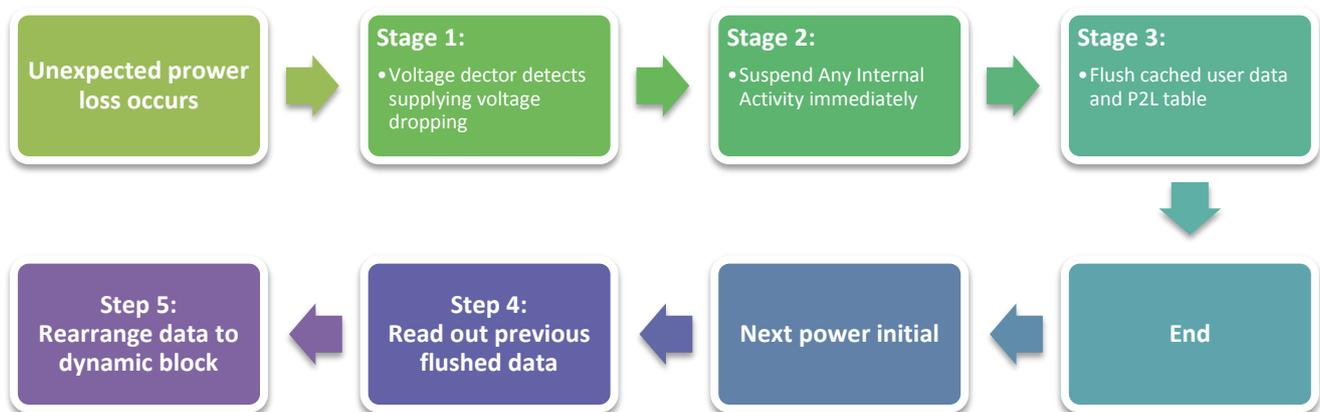
**Figure 2.** How SSD firmware mechanism handle unexpected power loss
