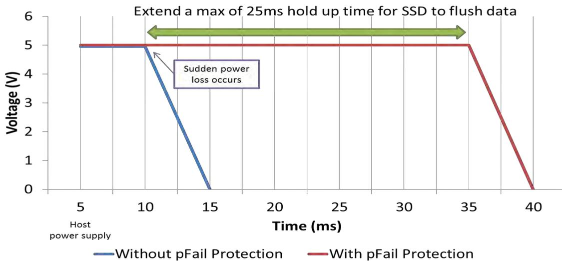
**Figure 3.** Hold up time for when unexpected power loss occurs
